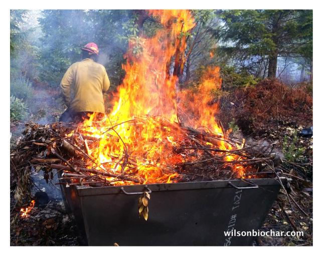
Designed by Wilson Biochar Associates for use in forestry to convert burn piles to biochar.
